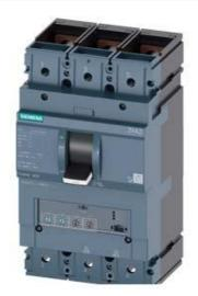
CIRCUIT BREAKER 3VA2 IEC FRAME 400 BREAKING CAPACITY CLASS H ICU=85KA @ 415 V 3-POLE, LINE PROTECTION ETU330, LIG, IN=250A OVERLOAD PROTECTION IR=100A ...250A SHORT CIRCUIT PROTECTION II=1,5...12 X IN GROUND-FAULT-PROTECTION IG=0,2... 1 X IN, TG=0,1/0,3MS BUSBAR CONNECTION
