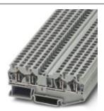
Feed-through terminal block, Connection method: Spring-cage connection, Cross section: 0.08 mm² - 6 mm², AWG: 28 - 10, Width: 6.2 mm, Color: gray, Mounting type: NS 35/7,5, NS 35/15
