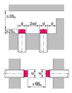
$\begin{array}{ll} S_n \, [mm] & \quad \text{Typ. operating range limit} \\ d & \quad \text{Diameter / distance} \end{array}$
