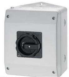
MASTER SWITCH 4-POLE IU=32, P/AC-23A AT 400V=11.5 KW 1 N TERMINAL ISOLATED SEALED, IP65 ROTARY MECHANISM BLACK METRIC THREAD
