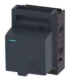
FUSE-SWITCH-DISCONNECTOR 3-POLE, NH000, 160A MOUNTING PLATE CONSTRUCTION COVER LEVEL 45 MM BOX TERMINAL FUSE MONITORING ELECTRONIC, EFM 10
