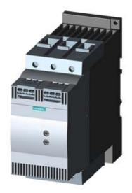
SIRIUS SOFT STARTER, SIZE S3, 80A, 45KW/400V, 40 DEGREES, 200-480V AC, 110-230V AC/DC, SPRING-LOADED TERMINALS
