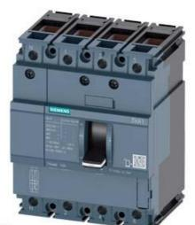
CIRCUIT BREAKER 3VA1 IEC FRAME 100 BREAKING CAPACITY CLASS B ICU=16KA @ 415 V 4-POLE, LINE PROTECTION TM210, FTFM, IN=16A OVERLOAD PROTECTION IR=16A FIXED SHORT CIRCUIT PROTECTION II=10 X IN NEUTRAL UNPROTECTED CABLE CONNECTION
