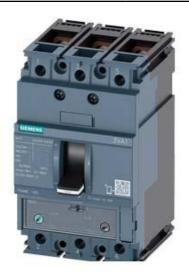
CIRCUIT BREAKER 3VA1 IEC FRAME 160 BREAKING CAPACITY CLASS N ICU=25KA @ 415 V 3-POLE, LINE PROTECTION TM240, ATAM, IN=20A OVERLOAD PROTECTION IR=14A ...20A SHORT CIRCUIT PROTECTION II=5...10 X IN BUSBAR CONNECTION
