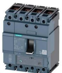
CIRCUIT BREAKER 3VA1 IEC FRAME 160 BREAKING CAPACITY CLASS H ICU=70KA @ 415 V 4-POLE, LINE PROTECTION TM240, ATAM, IN=50A OVERLOAD PROTECTION IR=35A ...50A SHORT CIRCUIT PROTECTION II=5 X IN NEUTRAL PROTECTION 100% BUSBAR CONNECTION
