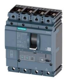
CIRCUIT BREAKER 3VA2 IEC FRAME 160 BREAKING CAPACITY CLASS C ICU=110KA @ 415 V 4POLE, LINE PROTECTION ETU320, LI, IN=63A OVERLOAD PROTECTION IR=25A ...63A SHORT CIRCUIT PROTECTION II=12 X IN NEUTRAL PROTECTION ADJUSTABLE(OFF,100%) BUSBAR CONNECTION
