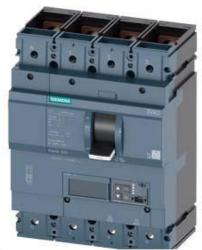
CIRCUIT BREAKER 3VA2 IEC FRAME 630 BREAKING CAPACITY CLASS C ICU=110KA @ 415 V 4-POLE, LINE PROTECTION ETU860, LSIG, IN=500A OVERLOAD PROTECTION IR=200A ...500A SHORT CIRCUIT PROTECTION ISD=0,6..10X IN, II=1,5..14X IN NEUTRAL PROTECTION ADJUSTABLE (OFF, UPTO 100%) GROUND-FAULT, SWITCHABLE IG=0,2... 1 X IN, TG=0,05-0,8MS BUSBAR CONNECTION
