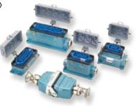
**revos** (a) multipole connectors are designed for special applications in hazardous areas. Their use in zone 1 for intrinsic circuits has been approved by the BVS test institute. The housings for the multipole connectors are manufactured from die cast zinc alloy.
