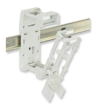
The mounting frames of the **revos** BASIC family are ideal for use in low-voltage switching systems. They are mounted directly to the 35x15 DIN rail according to DIN EN 50022 inside the control cabinet. Use of the DIN rail mounting frame on a 7.5 mm high DIN-rail  $35 \times 7.5$  in accordance with DIN EN 50022 is only possible if the installation space behind it is free.
