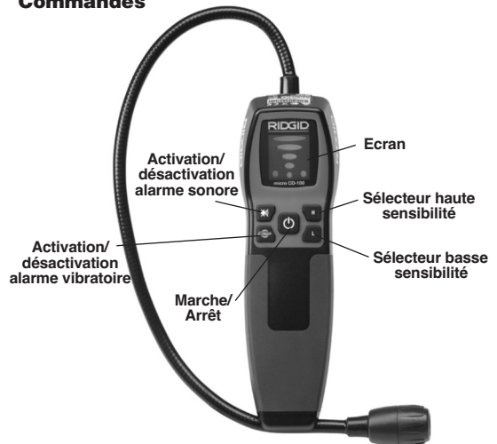
Figure 2 – Composants du micro CD-100
