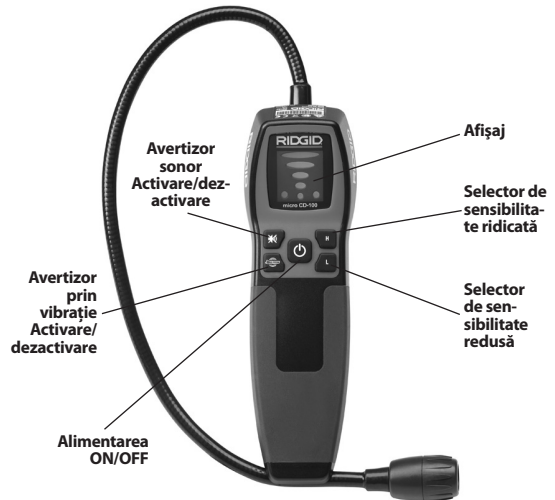
Figura 2 – Componentele micro CD-100
