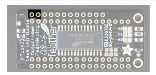
All LED control is done over I2C using the HT16K33 interface library. This means SDA and SCL must be connected, see above for those pins.
