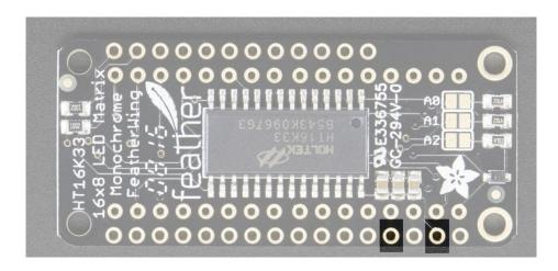
The LED matrix uses only the **3V** and **GND** pins for power and logic. Current draw depends on how many LEDs are lit but you can approximate it as about 120mA for most uses.
