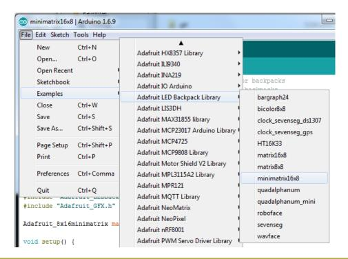
Note that the normal "matrix16x8" demo wont work the way you want because the matrix alignment is different on the Feather!
