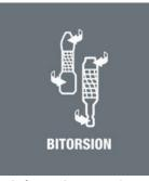
Peak forces that occur in power tool applications often result in premature wear of bits or damage to the screw head. This usually occurs during initial power-up and the when the screw comes to a Screwdriving could standstill. become more productive and safer if these peak loads could be minimised. The Wera BiTorsion system prevents premature wear. The service life of the tool is extended and the productivity of power tool applications significantly increased.
