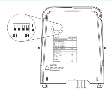
Configure the device in the following way:
