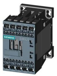
COUPLING CONTACTOR RELAY RAIL, 2NO+2NC, DC 24V, 0.7...1.25\*US, VARISTOR INTEGRATED, SZ S00, SPRING-LOADED TERMINAL
