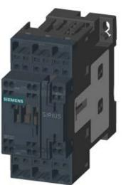
CONTACTOR, AC-3, 11KW/400V, 1NO+1NC, DC 125V, 3-POLE, SZ S0 SPRING-LOADED TERMINAL
