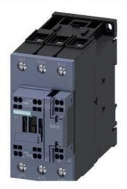
CONTACTOR,AC3:30KW/400V, 1NO+1NC, 175-280V AC/DC, WITH VARISTOR, 3-POLE, SIZE S2, SPRING-TYPE TERMINAL
