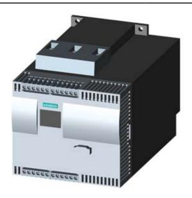
SIRIUS SOFT STARTER, VALUES WITH 575 V, 50 DEG., STANDARD: 42A, 30HP, INSIDE-DELTA CIRCUIT 3: 73A, 60HP, 400-690 V AC, 115 V AC, SCREW TERMINALS
