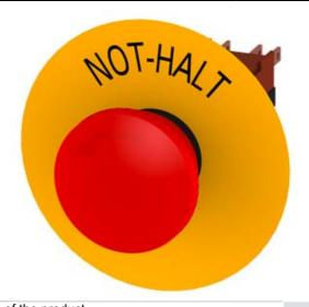
EMERGENCY-STOP MUSHROOM PUSHBUTTON, 16MM, ROUND, PLASTIC, RED, LATCHING, ROTATE-TO-UNLATCH MECHANISM, 1NC, WITH YELLOW BACKING PLATE, INSCRIPTION EMERGENCY-STOP
