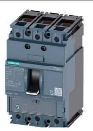
CIRCUIT BREAKER 3VA1 IEC FRAME 160 BREAKING CAPACITY CLASS M ICU=55KA @ 415 V 3-POLE, LINE PROTECTION TM220, ATFM, IN=25A OVERLOAD PROTECTION IR=17,5A ...25A SHORT CIRCUIT PROTECTION II=10 X IN CABLE CONNECTION
