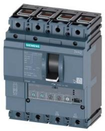
CIRCUIT BREAKER 3VA2 IEC FRAME 100 BREAKING CAPACITY CLASS H ICU=85KA @ 415 V 4POLE, LINE PROTECTION ETU350, LSI, IN=40A OVERLOAD PROTECTION IR=16A ...40A SHORT CIRCUIT PROTECTION ISD=1,5... 10 X IR, II=12 X IN NEUTRAL PROTECTION ADJUSTABLE(OFF,100%) CABLE CONNECTION
