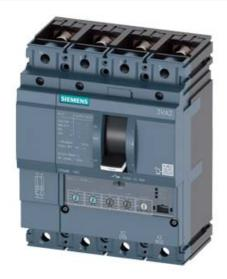
CIRCUIT BREAKER 3VA2 IEC FRAME 160 BREAKING CAPACITY CLASS H ICU=85KA @ 415 V 4POLE, LINE PROTECTION ETU350, LSI, IN=25A OVERLOAD PROTECTION IR=10A ...25A SHORT CIRCUIT PROTECTION ISD=1,5... 10 X IR, II=12 X IN NEUTRAL PROTECTION ADJUSTABLE(OFF,100%) BUSBAR CONNECTION
