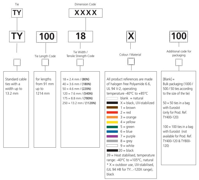
Note: Nylon (Polyamide) is inherently susceptible to environmental conditions. Ty-Fast® cable ties are moisturised to optimum performance levels at machineside and should be stored in cool dry areas out of direct sunlight. Cable ties are packaged in plastic bags to contain moisture and should remain sealed until ready for use.
