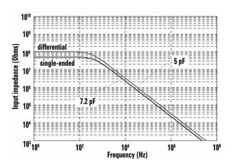
Figure 14. Input impedance vs. Frequency of N2891A
