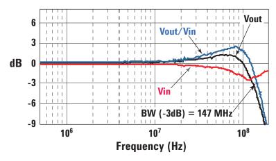
Figure 4. Vout/Vin vs. frequency response of N2790A
