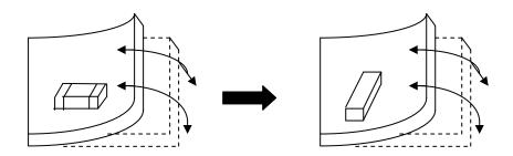
(2) Component layout close to board separation point. Susceptibility to stress in the order: A > C > B = D
