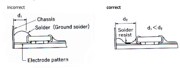
(3) Placing leaded components after chip component.
