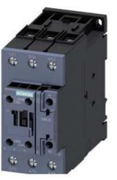
CONTACTOR,AC3:18.5KW/400V, 1NO+1NC, 20-33V AC/DC, WITH VARISTOR, 3-POLE, SIZE S2, SCREW TERMINAL
