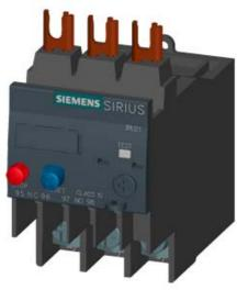
OVERLOAD RELAY 34...40 A FOR MOTOR PROTECTION SZ S0, CLASS 10, F. MOUNTING ONTO CONTACTOR MAIN CIRCUIT: RING CABLE LUG AUX. CIRCUIT: RING CABLE LUG MANUAL-AUTOMATIC-RESET
