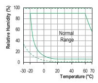
Long term exposure to humidity levels outside of the 'normal' range may temporarily offset RH measurements (±3%RH after 60 hours). Once returned to less extreme conditions the device will slowly return towards calibration state.
