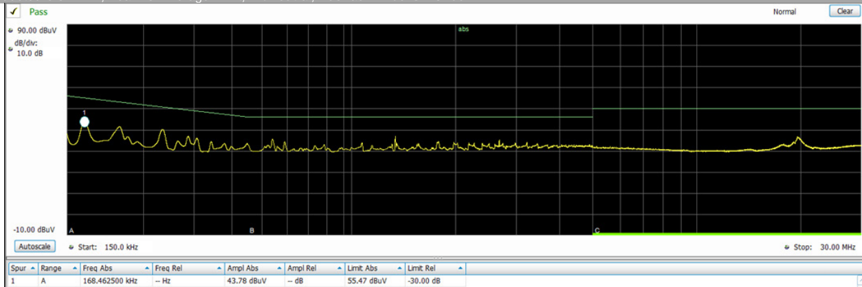
EMI; Conducted CISPR 22; Peak vs. Average Limit; L1; 208Vac 24Vdc @ 25A dc
