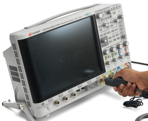
Figure 4 Connecting the Probe to the Oscilloscope
