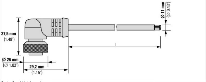
Supply cable, prefabricated on one side
