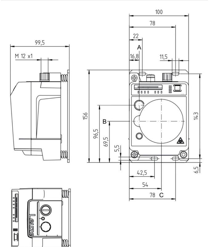
A Center axis of transmitter and alignment laser B Center axis of transmitter and receiver
