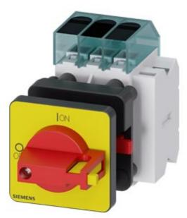
Switch disconnector 3LD3, main switch 3-polig, lu 40A operational switch at AC-23 A at 400 V 15,0 kW front mounted Base mounting with center-hole 22,5 mm knob-operated mechanism red/yellow 48 x 48 mm with auxiliary 1NO+1NC
