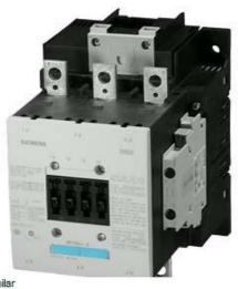
CONTACTOR, 75KW/400V/AC-3, AC(40...60HZ)/DC OPERATION UC 220...240V AUXIL. CONTACTS 2NO+2NC 3-POLE, SIZE S6 BAR CONNECTIONS CONVENTIONAL OPERATING MECHAN. SCREW TERMINAL
