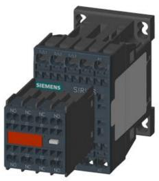
CONTACTOR, AC-3, 3KW/400V, 2NO+2NC, DC 24V, 3-POLE, SZ S00 SPRING-LOADED TERMINAL PERMANENT AUX. SWITCH FOR SUVA **APPLICATIONS**
