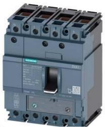
CIRCUIT BREAKER 3VA1 IEC FRAME 160 BREAKING CAPACITY CLASS M ICU=55KA @ 415 V 4-POLE, LINE PROTECTION TM240, ATAM, IN=63A OVERLOAD PROTECTION IR=44,1A ...63A SHORT CIRCUIT PROTECTION II=5...10 X IN NEUTRAL PROTECTION 100% CABLE CONNECTION
