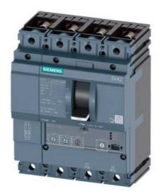
CIRCUIT BREAKER 3VA2 IEC FRAME 160 BREAKING CAPACITY CLASS M ICU=55KA @ 415 V 4POLE, LINE PROTECTION ETU320, LI, IN=160A OVERLOAD PROTECTION IR=64A ...160A SHORT CIRCUIT PROTECTION II=10 X IN NEUTRAL PROTECTION ADJUSTABLE(OFF,50%,100%) BUSBAR CONNECTION
