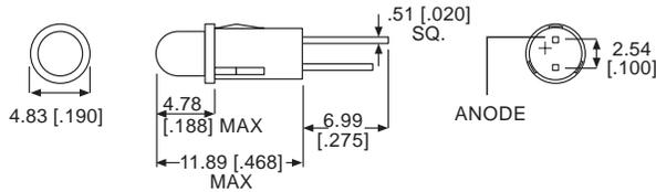
26 AWG 6" WIRE LEADS – TERMINAL OPTION 3 FOR 6" TERMINAL OPTION 7 FOR 14"
