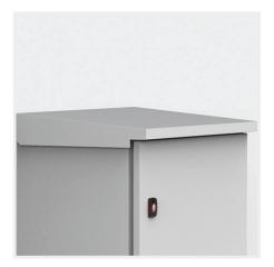
**Omschrijving:** To be fitted as an outdoor shelter on single mounted enclosures. The roof is slightly sloped and has a dripstrip. Machining is required. It increases the enclosure dimension in H:60 mm, D:20 mm and W:20 mm.
