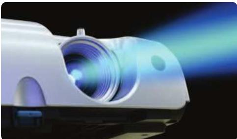
High-efficacy LEDs enable long operating life in portable projectors. Common-anode connected RGB LEDs are used to reduce wiring and ensure low thermal impedances for the LED. This requires the use of four high-efficiency, low-voltage LED drivers.
