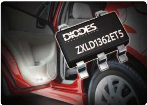
Door safety lamps usually use just one high-brightness LED so a simple buck converter is typically used. The lamp operates directly off the battery, requiring the driver to withstand load dump as well as meeting AEC-Q100 automotive quality requirements.
