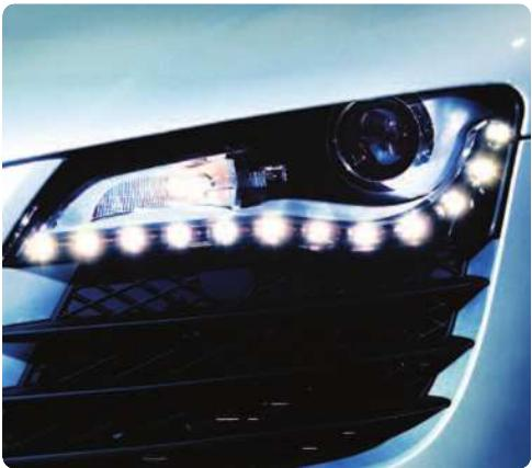
Due to the variation in battery voltage and the number of LEDs used, buck-boost configurations are commonly used in daytime running lights.
