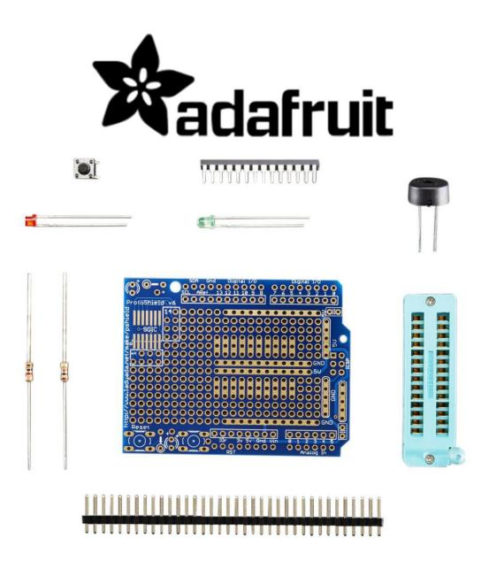
This shield kit pack will allow you to turn any Arduino into an AVR chip burner! It is specifically designed for people who want to program Atmega328P's to turn them into Arduino bootloader chips using an AVR-ISP sketch, but it can also be used to make a 'standalone' AVR ISP programmer – so that you can program blank chips without a computer! A blank ATmega328P DIP chip is included so you can get to programming immediately! Comes with:
