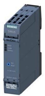
Thermistor motor prot. relay Device for warning and tripping 22.5 mm enclosure Spring-type terminals 1 NO contact + 1 CO contact US = 24 V-240 V AC/DC Manual/Auto/Remote RESET with ATEX certification 3 LEDs (READY/WARNING/TRIPPED) Protective separation Test/Reset button Open-circuit monitoring Short-circuit monitoring Non-volatile 2 separate PTC sensor circuits
