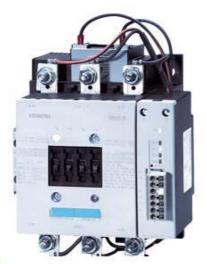
CONTACTOR, 55KW/400V/AC-3 AC(40...60HZ)/DC OPERATION UC 96-127V AUXILIARY CONTACTS 1NO+1NC 3-POLE, SIZE S6 BAR CONNECTIONS ELECTRONIC OPERATING MECHANISM WITH PLC/SIMOCODE INTERFACE AND REMAIN. LIFETIME INDICATOR
