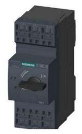
CIRCUIT-BREAKER SZ S0, FOR MOTOR PROTECTION, CLASS 10, A-REL. 0.55...0.8A, N-REL. 10A SPRING-L. CONNECTION STANDARD SW. CAPACITY
