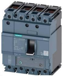
CIRCUIT BREAKER 3VA1 IEC FRAME 160 BREAKING CAPACITY CLASS N ICU=25KA @ 415 V 4-POLE, LINE PROTECTION TM240, ATAM, IN=32A OVERLOAD PROTECTION IR=22,4A ...32A SHORT CIRCUIT PROTECTION II=5...10 X IN NEUTRAL PROTECTION 100% CABLE CONNECTION
