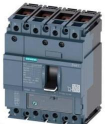
CIRCUIT BREAKER 3VA1 IEC FRAME 160 BREAKING CAPACITY CLASS S ICU=36KA @ 415 V 4-POLE, LINE PROTECTION TM220, ATFM, IN=32A OVERLOAD PROTECTION IR=22,4A ...32A SHORT CIRCUIT PROTECTION II=10 X IN NEUTRAL UNPROTECTED BUSBAR CONNECTION
