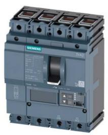
CIRCUIT BREAKER 3VA2 IEC FRAME 100 BREAKING CAPACITY CLASS H ICU=85KA @ 415 V 4POLE, LINE PROTECTION ETU550, LSI, IN=40A OVERLOAD PROTECTION IR=16A ...40A SHORT CIRCUIT PROTECTION ISD=0,6..10X IN, II=1,5..12X IN NEUTRAL PROTECTION ADJUSTABLE (OFF, UPTO 160%) CABLE CONNECTION
