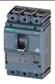
CIRCUIT BREAKER 3VA2 IEC FRAME 160 BREAKING CAPACITY CLASS M ICU=55KA @ 415 V 3POLE, LINE PROTECTION ETU330, LIG, IN=160A OVERLOAD PROTECTION IR=64A ...160A SHORT CIRCUIT PROTECTION II=1,5...10 X IN GROUNDFAULTPROTECTION IG=0,2... 1 X IN, TG=0,1/0,3MS CABLE CONNECTION
